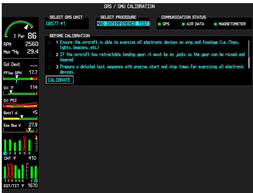
**Figure 7-11. Magnetometer Interference Test**
